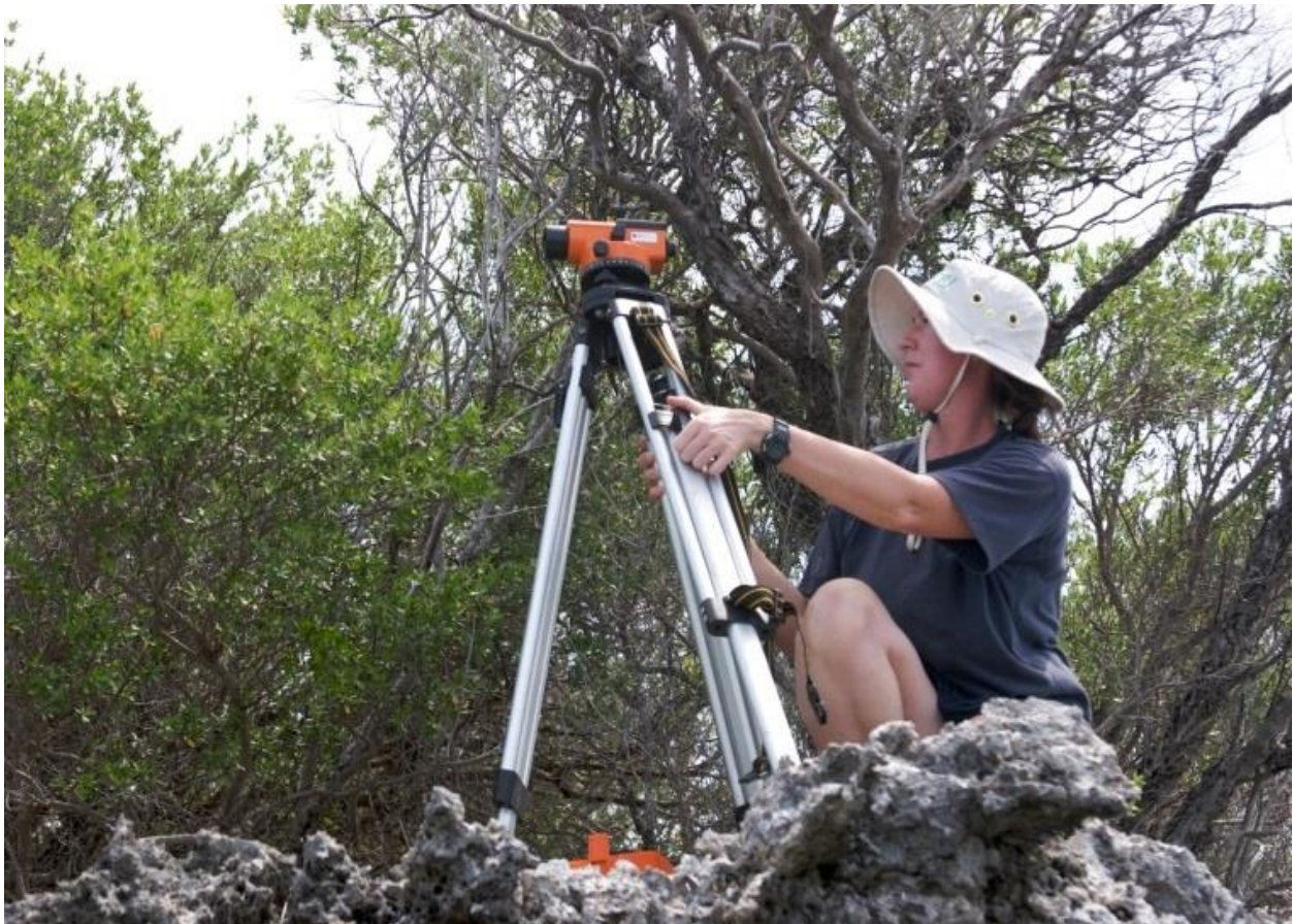
Figure 3. Conducting semi-automatic level surveys to calculate relative height differences between benchmarks.
