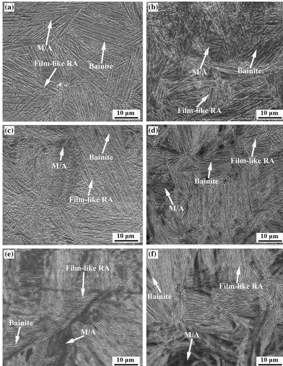
**Fig. 3** The microstructure of different samples austempered at different temperatures for 30 h: **a** Ni-free steel, 200 °C; **b** Ni-added steel, 200 °C; **c** Ni-free steel, 220 °C; **d** Ni-added steel, 220 °C; **e** Ni-free steel, 250 °C; **f** Ni-added steel, 250 °C
