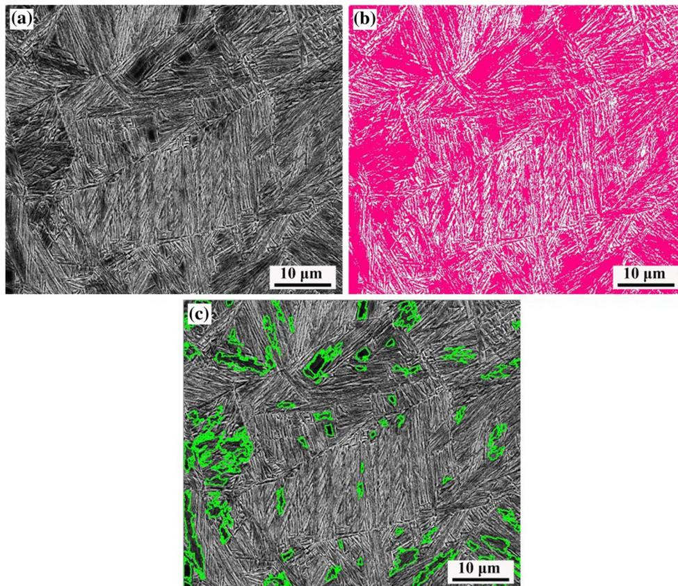
**Fig. 2** The example to show how to calculate the volume fraction of bainite: **a** the original micrograph; **b** the darker areas in **a** are colored pink; **c** the darker blocky places are manually marked
