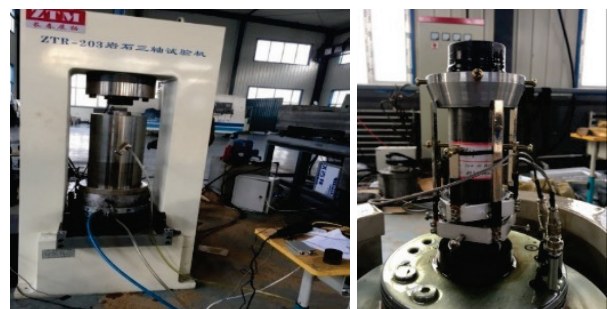
Figure 1 ZTR-203 electro-hydraulic servo rock three-axis test system
