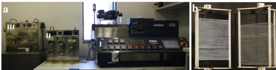
Figure 3.4: (a) melt spinning setup, I: twin-screw melt extrusion, II: stretching unit and III: winding unit, and (b) left: pure and right: LCGO-coated LDPE powder.
