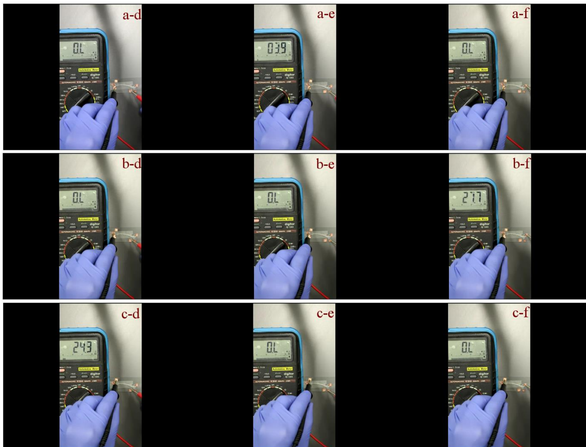
Figure 6.5: connectivity test for braid structure showing that each end of an electrode in one side (a-c in Figure 6.4 ) is connected to only one end to the other side (d-f in Figure 6.4 )
