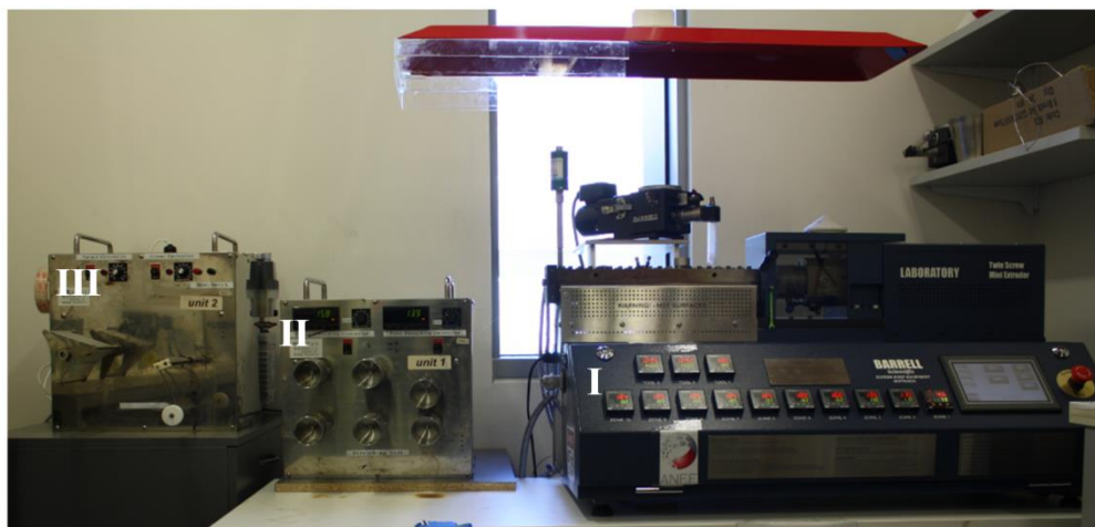
Figure 2.2: melt spinning setup, I: twin-screw melt extrusion, II: stretching unit and III: winding unit
