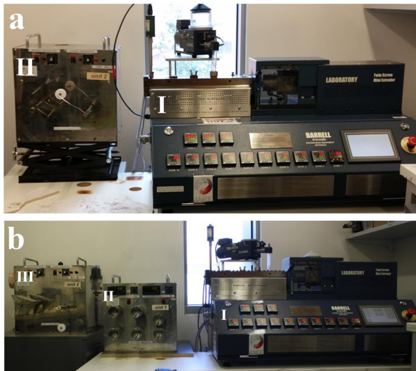
Figure 4.1: (a) melt spinning setup for making (a) undrawn LDPE fibres, I: twin-screw melt extrusion, II: winding unit and (b) drawn LDPE fibres, I: twin-screw melt extrusion, II: stretching unit and III: winding unit
