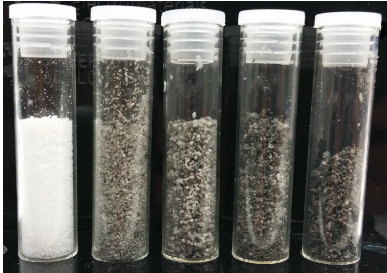
Figure 3.1: left to right: LDPE, 0.5, 1, 2 and 5 w/w% LCGO/LDPE powders
