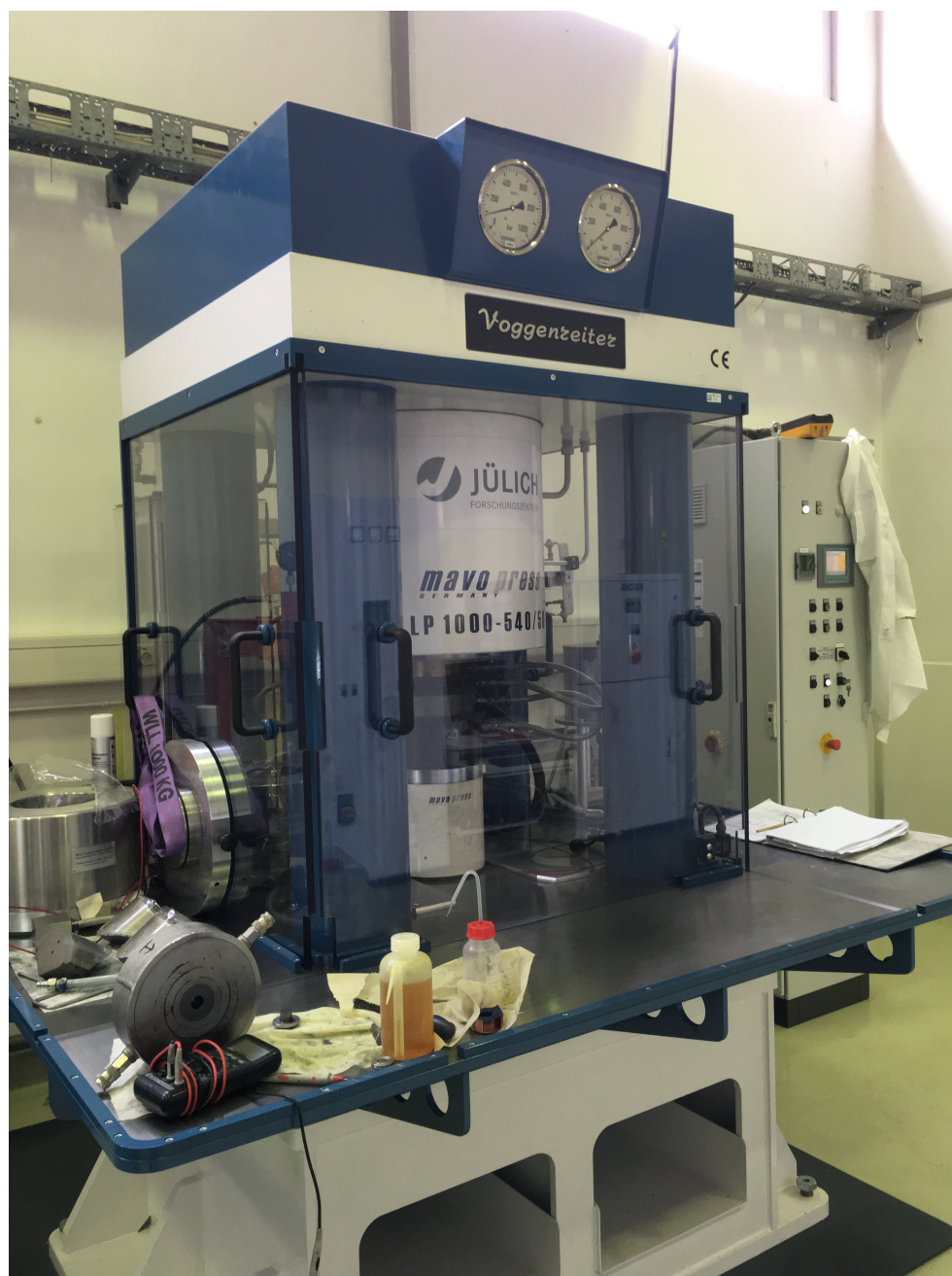
FIGURE 6.1: Voggenreiter LP 1000-540/50 high temperature high pressure apparatus installed at IEK-6, Forschungszentrum Jülich, Germany.
