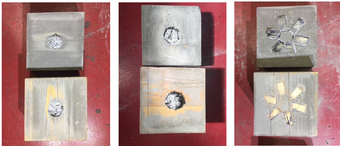
(a) (b) (c) Figure 3 Failure of the specimens: (a) C-N, (b) 40-N, and (c) 40-NN.
