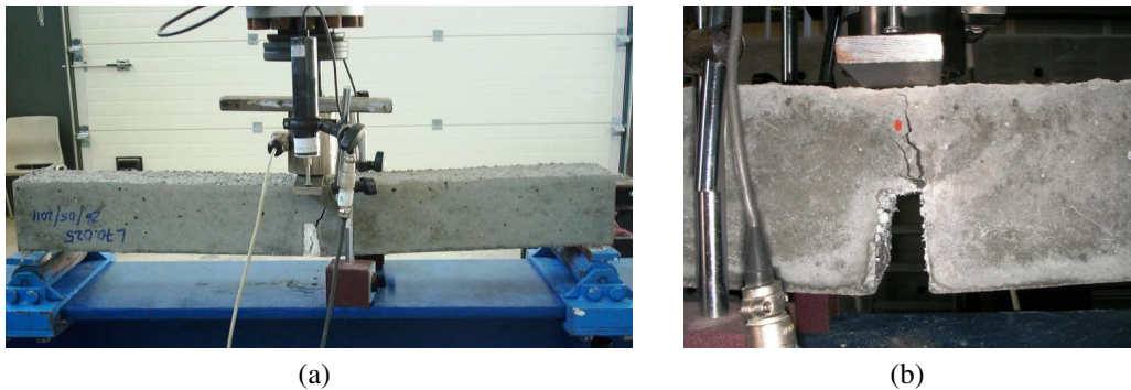
Figure 3: Three point FRC bending beam: (a) test set-up; and (b) failure mechanism during a test.
