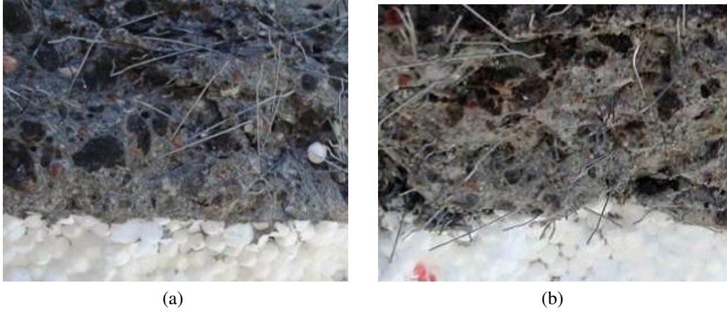
Figure 5: Three point FRC bending beam: fibre distribution on top of the notch for the specimens with 0.50% of steel fibres: (a) wrong distribution in one specimen; and (b) adequate distribution according to [26].
