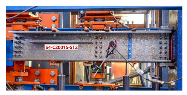
FIGURE 4.10. Test setup for beams with transverse web stiffener
