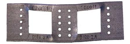
FIGURE 6.16. Failure mode on shear test on C20019-S120 member
