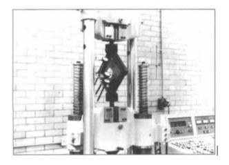
FIGURE 2.22. Shear tests on plates with holes (Narayanan & Der-Avanessian, 1985)
