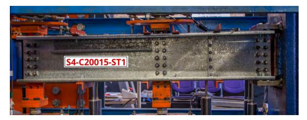
FIGURE 4.11. Failure mode of the test with the UA20x25x2.4 transverse stiffener
