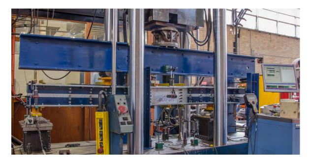
FIGURE 3.18. Overall test configuration for a plain channel member
