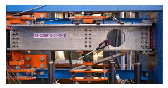
FIGURE 4.3. Test configuration for beams with web holes
