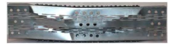
FIGURE 2.25. Failure mode of slotted web in shear
