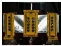
b) Shear failure mode of a beam with an aspect ratio of 1.0
