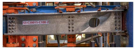
(b) Circular hole with a diameter of  $100 \ mm$
