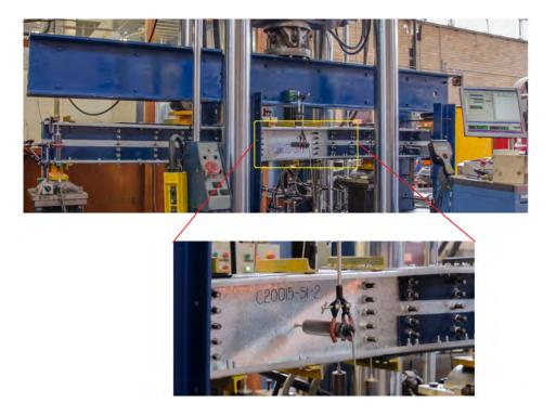
FIGURE 3.20. Test configuration and shear failure mode of plain channel test segment
