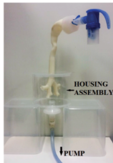
Figure 1. Physical test apparatus used to assess total airway deposition.
