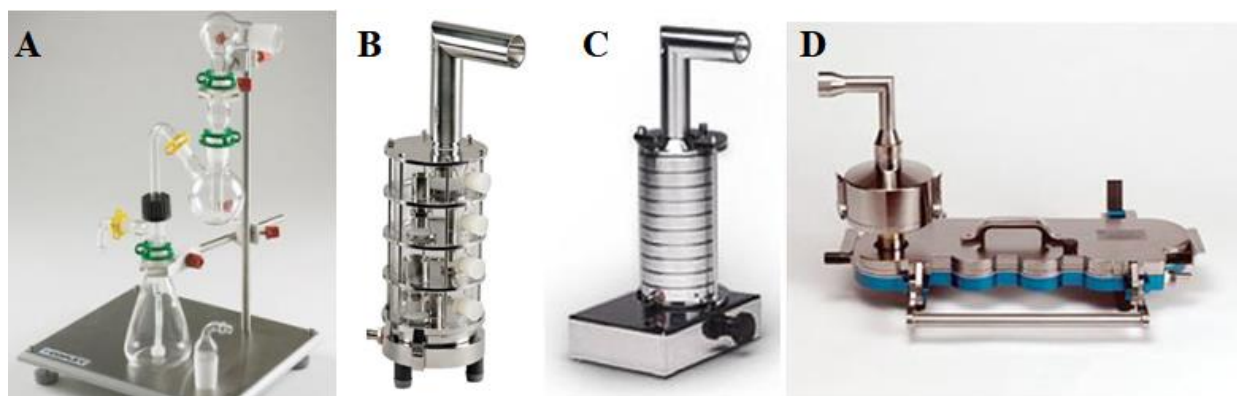
Figure 2. List of compendial apparatuses used for routine sizing characterisation, showing the: A) Two-Stage Liquid Impinger, B) Multi-Stage Liquid Impinger, C) Andersen Cascade Impactor, and D) Next Generation Impactor [45].
