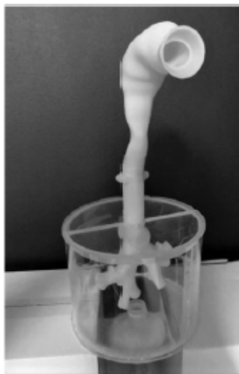
FIG. 2. Physical setup of the modified airway model (MOD#2) used to assess in vitro airway deposition of nebulized CIP-HCL. CIP-HCL, ciprofloxacin-hydrochloride.
