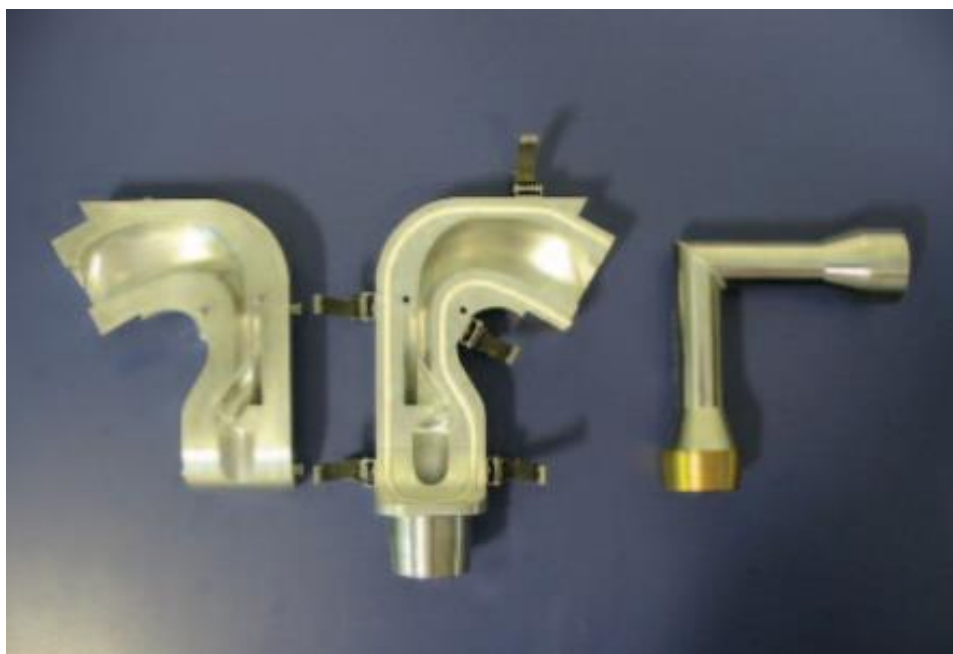
Figure 5. The Alberta Idealised Throat (left, in open form) and the USP/Ph. Eur induction port (right) [28].
