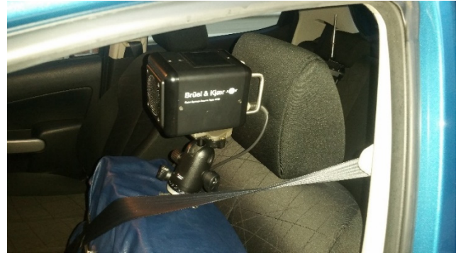
Figure 2. The positioning of speech source (4720) and receiver (Earthwork M30) inside the car
