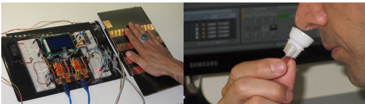
Picture 1. GSR sonification hardware and associated sensors. The south pole of the magnet on the right hand is directed downwards to close the linear magnetic switch.
