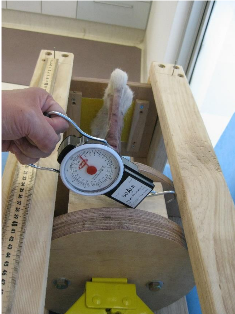
Figure 4-10: A rotation force was applied to identify the torque required for foot slippage. This value would also include frictional forces in the system and was quantified using a spring-loaded scale.
