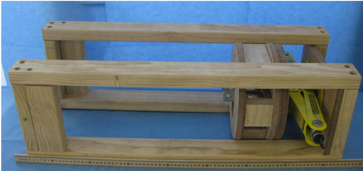
Figure 4-5: The redesigned jig (jig2) with a frame that comprised 4 beams of structural pine and housed the proximal limb restraint and foot plate (not shown above). Wood was selected as the construction material as it was inexpensive, radiolucent and easy to work with. The open sides allow the operator to visualise the limb position from two orthogonal positions.
