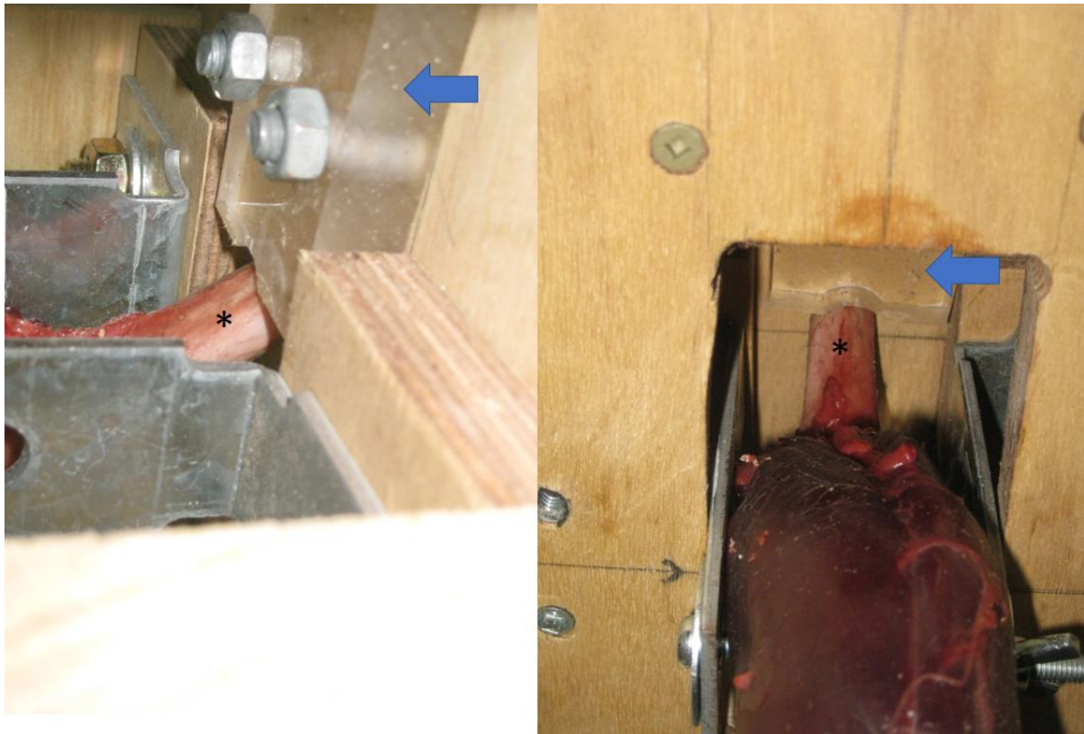
Figure 4-17: shows a side view (left) and view from distal to proximal (right) of the redesigned proximal limb restraint. The femoral block (blue arrow) rests caudal to the proximal femur (Asterix). As the limb is loaded and gastrocnemius tensioned, a force pulling the femur caudally into flexion is created. The femoral block resists this force.
