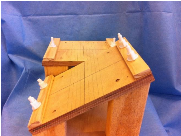
Figure 4-13: shows the two foot plates. The centre of both the flat plate (behind) and sloped plate (front) are marked. The plastic screws and wooden strips allow the non slip surface to be firmly attached to the plate, without creating any imaging artifacts.
