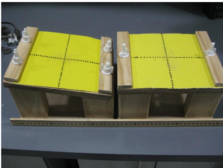
Figure 4-14: shows the flat (right) and 10 degree sloping foot plate(left). Both have a non-slip surface attached and the centre of the plate marked to facilitate foot placement
