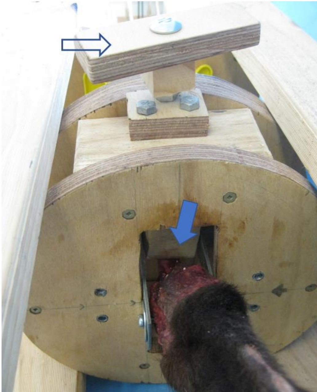
Figure 4-18: shows further modifications to the proximal limb restraint. The femoral block (blue arrow) positioned to resist stifle flexion is now larger and a bolt is positioned behind the block to prevent slippage of the block and permit easy alteration of femoral block position. A handle (open arrow) was secure to the end of the bolt to allow convenient adjustment to the craniocaudal position of the femoral block.
