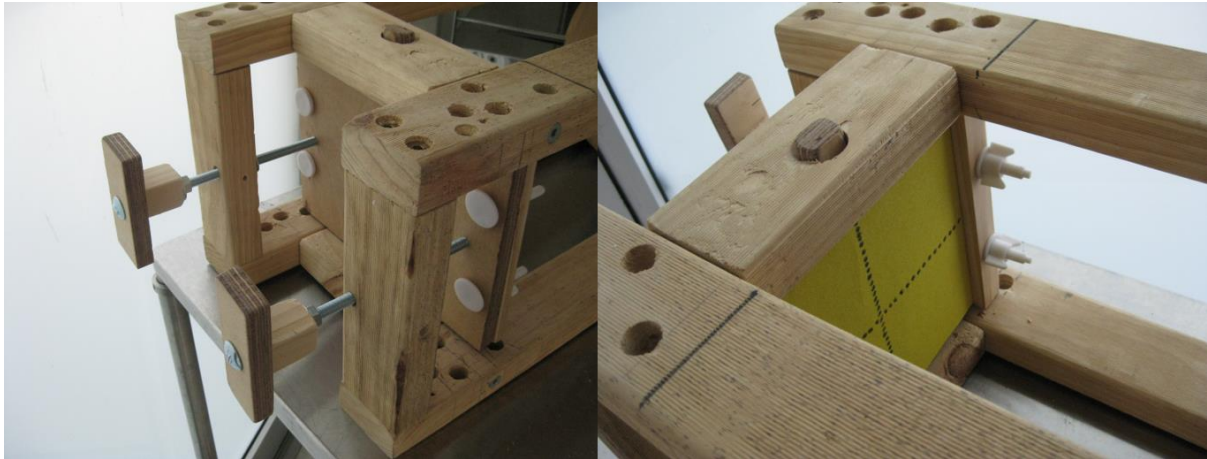
Figure 4-16: Left: the underside of the foot plate, which is held in place with two large bolts. These bolts can be adjusted to produce fine movements and hence infinite plate angles. Right: the top surface of the foot plate shows the non-slip surface with the centre of the plate marked.
