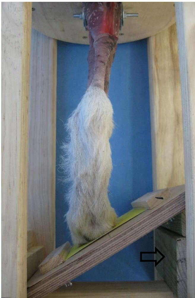
Figure 4-9: shows the slope created by placement of wooden blocks (open arrow) under the foot plate. The maximal angle was recorded before foot slippage
