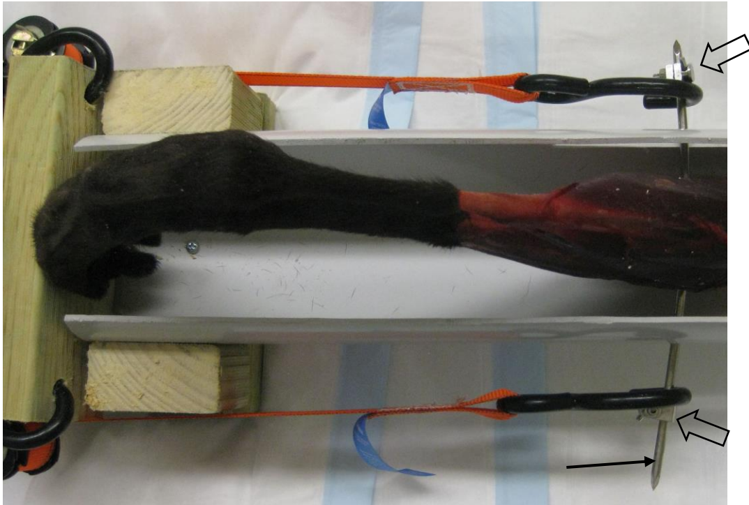
Figure 4-4: View of the limb loading jig from the caudal aspect of the limb. The trans-tibial pin is seen to plastically deform (arrow). External skeletal fixator clamps (open arrows) were attached to the trans-tibial pin to prevent slippage of the strap hooks
