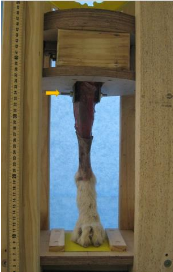
Figure 4-8: Cranial view of the jig with limb loaded. The proximal tibia is secured to the jig with a 6mm threaded bolt positioned through a previously drilled bone tunnel (yellow arrow). The distance between the aluminium brackets was customised to decrease the distance between bracket and the limb. This would reduce bending forces on the trans-tibial pin.
