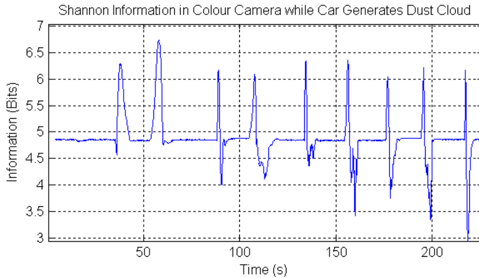
Figure 5.2: The entropy or average Shannon information of images in a colour video sequence, in which a vehicle repeatedly drives across the camera viewpoint along a dirt road. The appearance of the vehicle is relatively informative, whereas the dust cloud that follows is very uninformative. The vehicle drives faster by approximately 10km/h each time, creating a larger dust cloud and a corresponding decrease in information content. The first two passes at 40 and 59 seconds generate so little dust that the camera entropy is unaffected.
