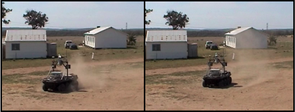
Figure 5.26: The two images have been selected from video footage of the real-time dust experiment, to illustrate the dust that is stirred into the air as the vehicle turns. This volume of dust is enough to reduce the ranges that are reported by the laser range scanner, causing the perception system to consider the region to be non-traversable. The dust model in Equation 5.7 that was learnt from the classification data is used in real-time to filter the laser sensor measurements. Measurements that are more likely to be affected by dust than not, are discarded to prevent them from being perceived as an obstacle to the vehicle.
