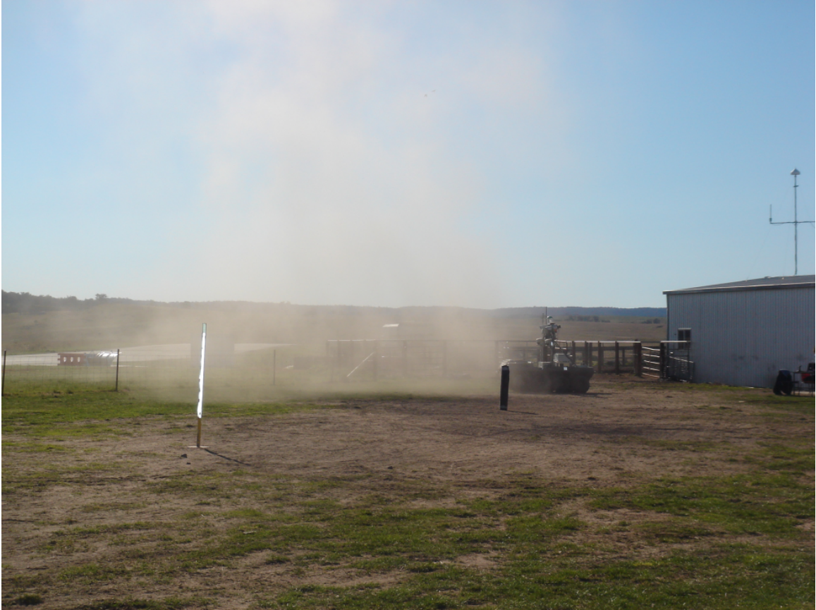
Figure 5.25: This eroded section of ground is used as a ‘worst case’ test site for the real-time performance of the dust filter. The figure shows the ability of the wind to raise significant volumes of dust into the air, independently of the vehicle. The interaction between the vehicle’s tyres and the ground also causes dust to be stirred in the vicinity of the vehicle as can be seen in Figure 5.26. Airborne dust is the primary cause of sensor failure for the laser range scanners in this type of outdoor environment.
