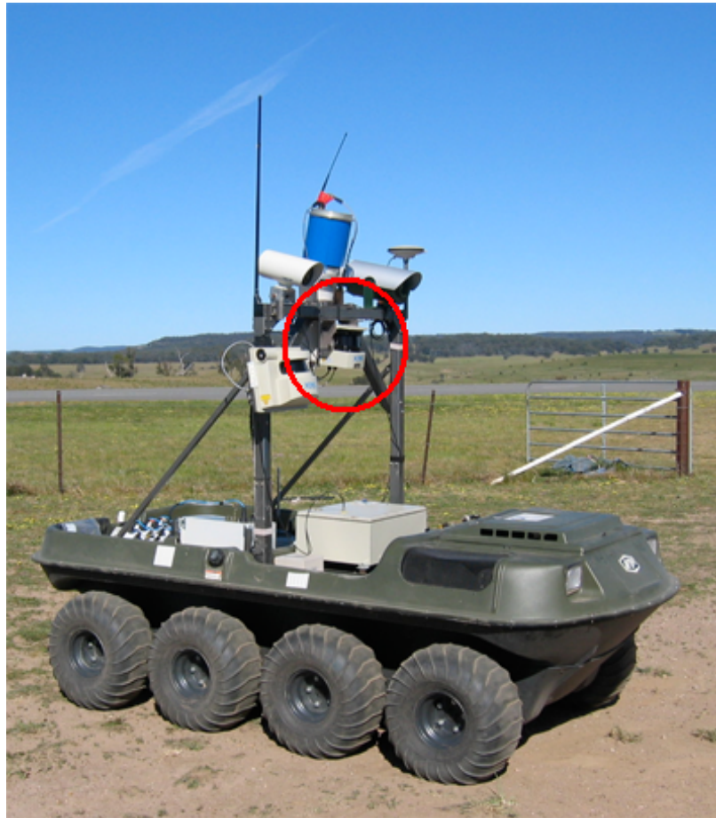
Figure 3.8: The CAS outdoor research demonstrator platform, with multiple sensors attached. The circled SICK LMS291 2D laser range scanner is used as the source of data for the this section. As shown, the laser is mounted at the top centre of the platform, looking forwards. The laser is pitched down 8 degrees from horizontal, and is mounted to align to the frame with zero roll and yaw.
