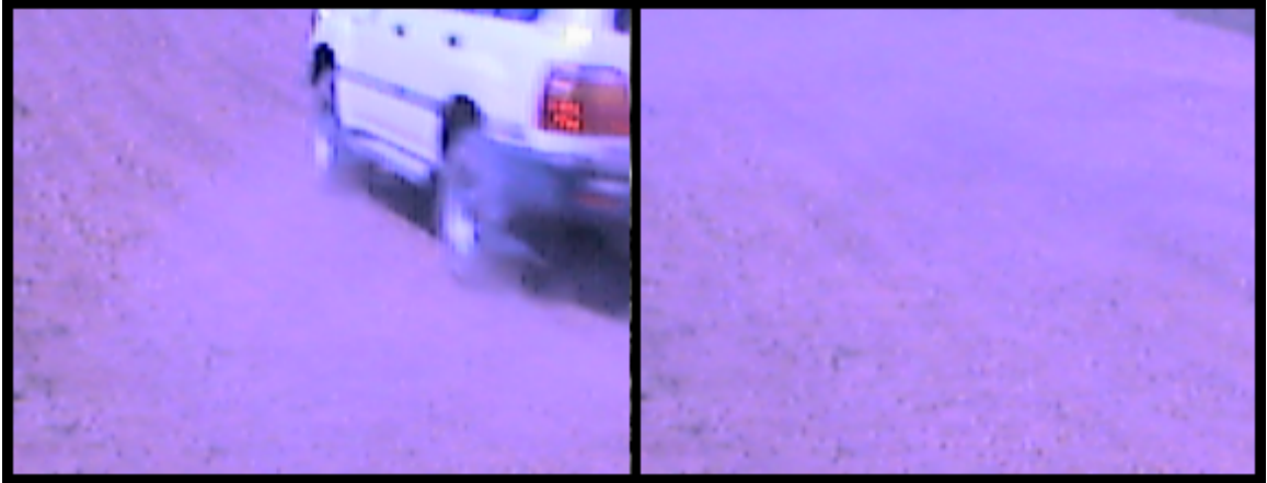
Figure 5.1: A vehicle is driven on a dirt road past the colour camera. The dust stirred behind the vehicle lingers in the atmosphere for several seconds, during which time the colour camera images appear washed out.
