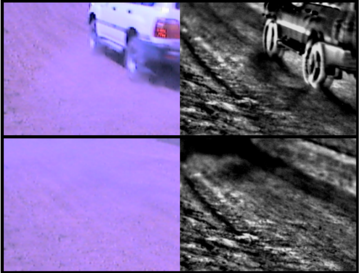
Figure 5.8: Two synchronised pairs of colour and thermal infrared camera images, shown after coarse alignment has been performed. Visibly the car is in the same place in both images, but because no intrinsic or extrinsic calibration has been done, the alignment quality may vary with the geometry of the environment. In the top image pair, a car can be seen driving across the scene. Moments later, the bottom pair shows the trail of dust behind the vehicle. The colour camera image appears to be more affected than the thermal image.
