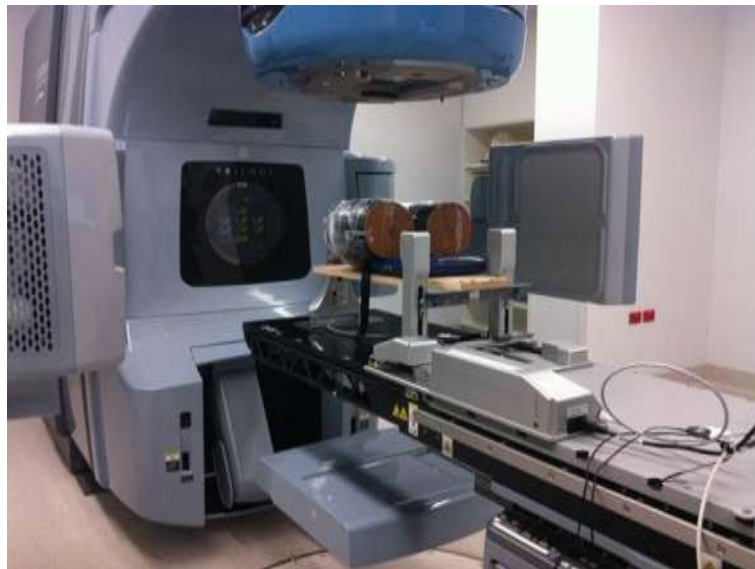
155 Figure 2. Setup of the Rando phantom for the QA tests. The Rando phantom was placed on an in-house modified wooden platform mounted to the HexaMotion. The HexaMotion translates the Rando phantom with programmed prostate trajectories during irradiation.
