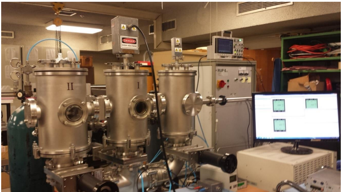
Figure 2.1: Photograph of plasma polymerization apparatus in the School of Physics used in this work. The cylindrical SS chamber was used here for PAC deposition and synthesis of nanoP 3 .
