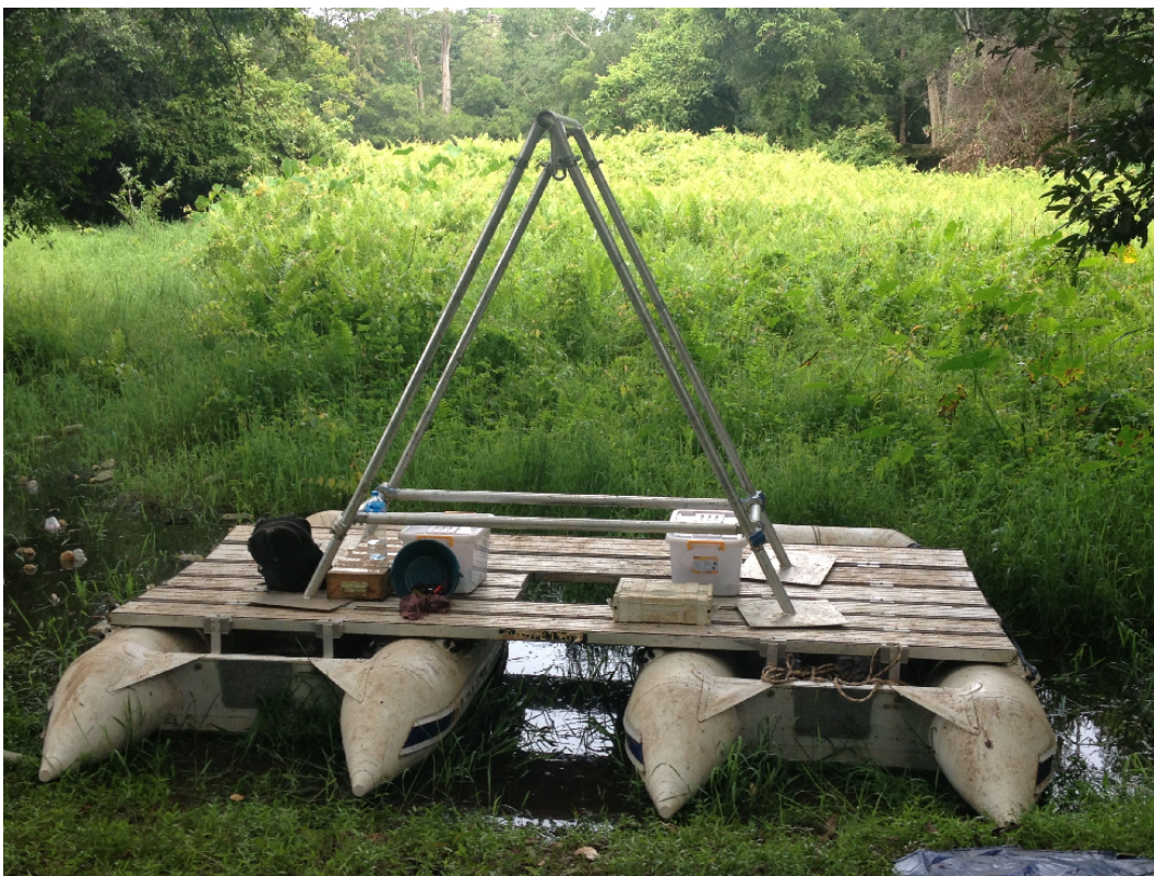
FIGURE 5.2: Coring platform, including two adjacent inflatable boats, aluminium platform and constructed aluminium frame. The percussion corer was subsequently suspended from the u-bolt below the apex of the frame.
