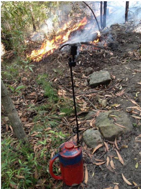
Figure 4.3 A drip torch used by the RFS in hazard reduction burning. Source: Lisa Maxwell, Blue Mountains Firewatch and Recovery Facebook page.
