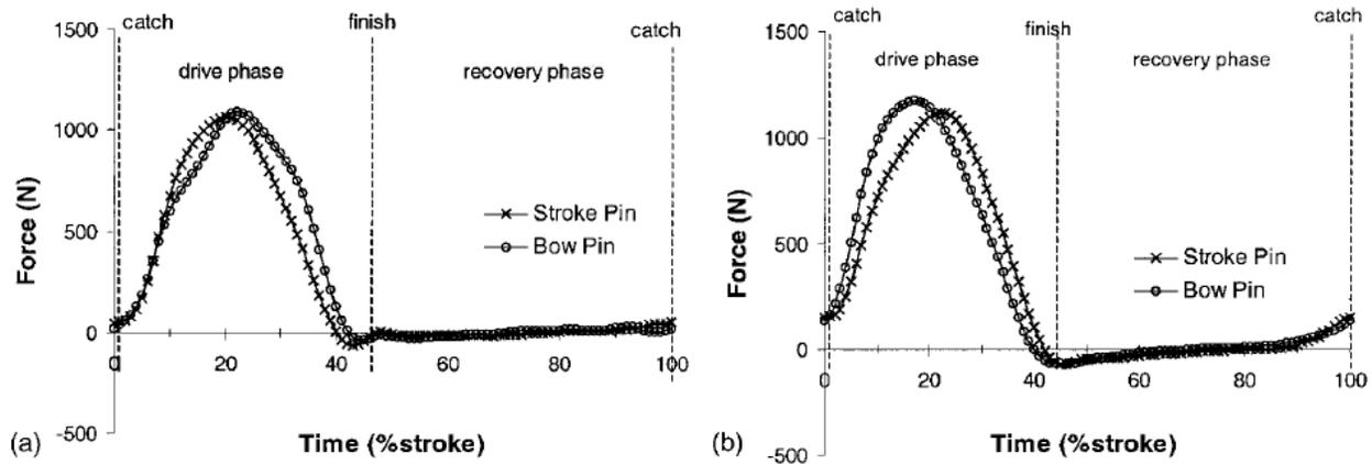
**Figure 3.** Example of force-percentage profiles in Smith and Loschner (2002). This figure depicts the relative timing between the stroke and bow pin propulsive forces in a pair for skilled (a) and less skilled (b) rowers. The curves are time-normalised and averaged data for 12 consecutive strokes at 30 strokes per minute.
