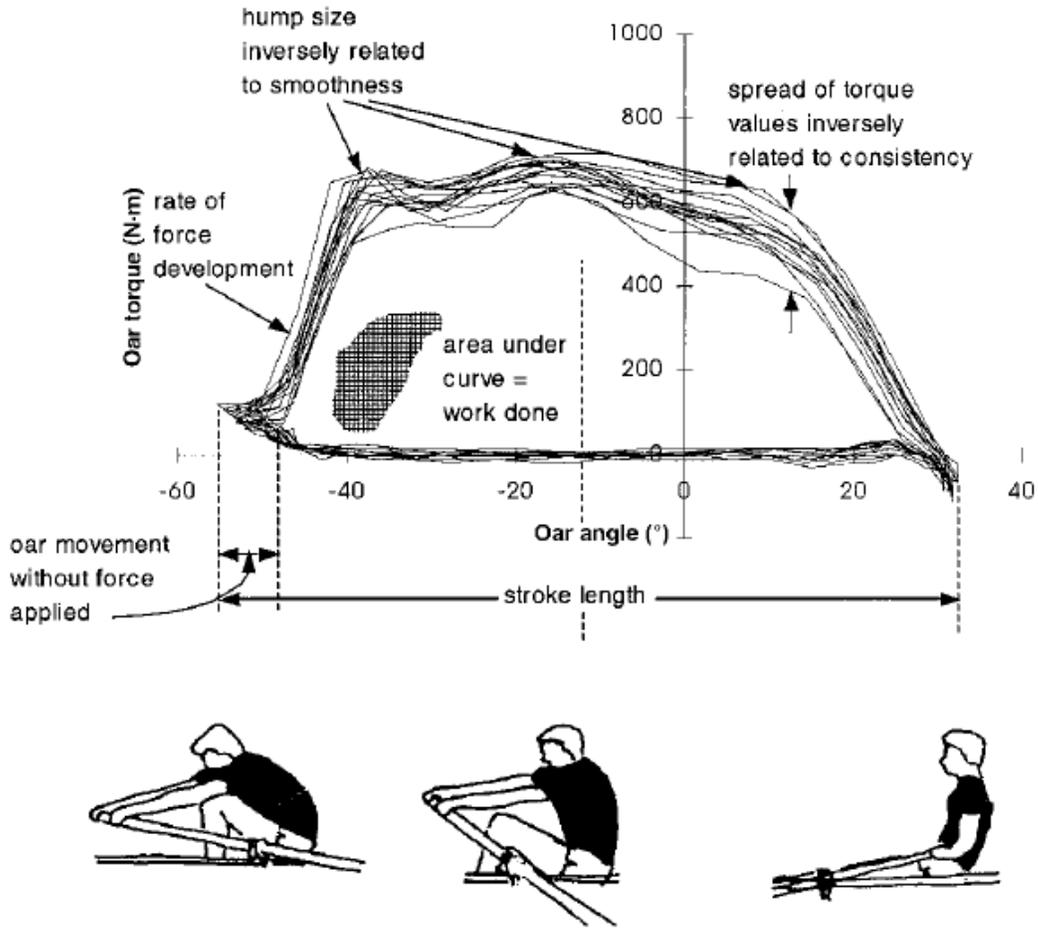
**Figure 4.** Example of force-angle profiles in Smith and Loschner (2002). This figure depicts a series of force-angle profiles of a club level rower. This graph also depicts a range of technical parameters that can be inferred from the shape characteristics of the force-angle profile.
