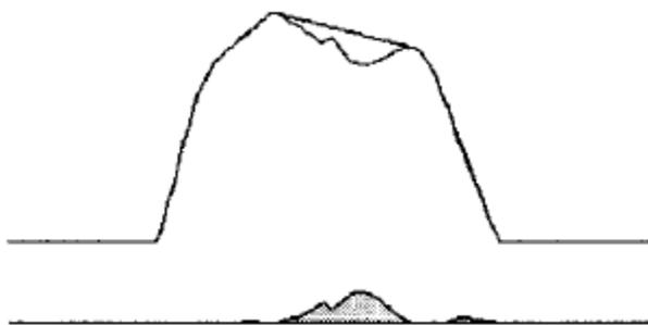
**Figure 5.** The smoothness measure as defined by Hill (2002). The shaded difference area relative to the force-time profile provides the value for smoothness, which in the present example is case 4%.
