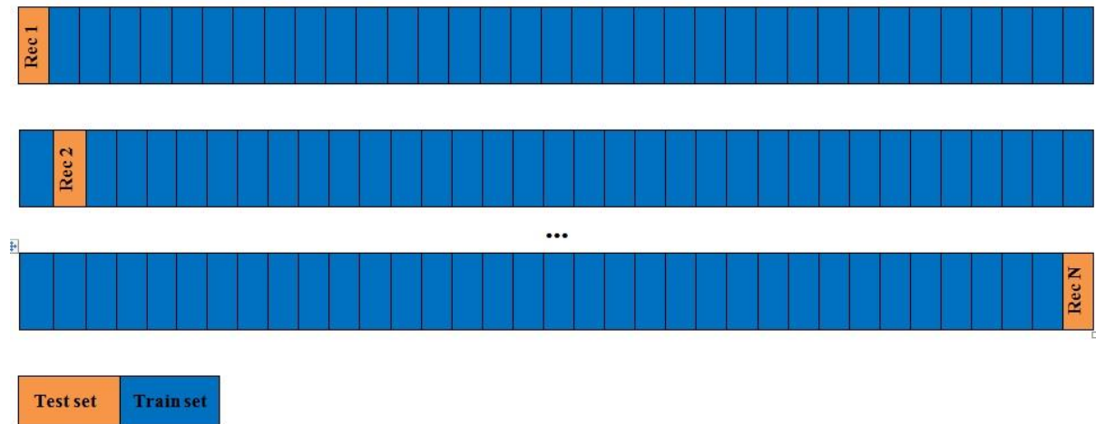
Figure 3.12. An illustration of leave-one-record-out cross validation for N recordings, with one record set to the test or validation set and the remaining recordings used as the training set in every iteration.
