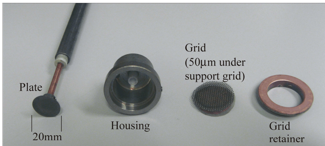
Figure 78 Components of the Retarding Field Energy Analyzer (RFEA) built for this project. With the exception of the plate (mild steel) and its mounting rod (copper), all metallic parts were made from stainless steel. The insulators were made from Teflon. The grid was in contact with and at the same potential as the housing which was connected to an external supply through a lead attached to the back of the housing. The copper on the grid retainer was the result of using the RFEA to measure the energy of copper ions in HiPIMS experiments. The housing was insulated from the plasma with a Teflon cover when in use.
