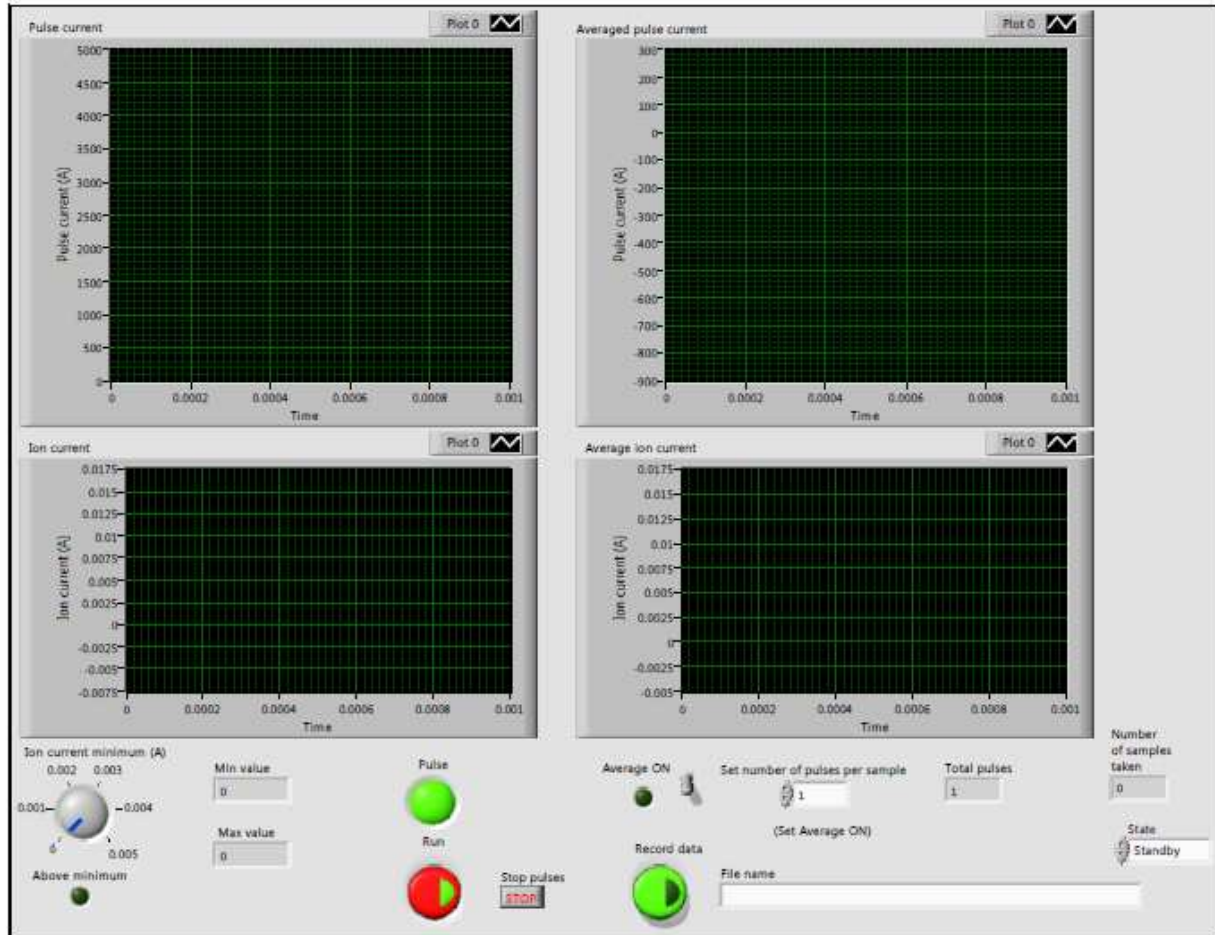
Figure 82 Front panel of the Labview virtual instrument used to control the magnetic reconnection experiment. Shown are four charts, the two on the left display the immediate measurements of pulse current and ion current, the two on the right display the average of successive measurements of pulse current and ion current. Controls on the left set the minimum threshold for recording an ion current, controls in the center run and stop experiments, controls on the right set the number of pulses for each experiment and record measurements.
