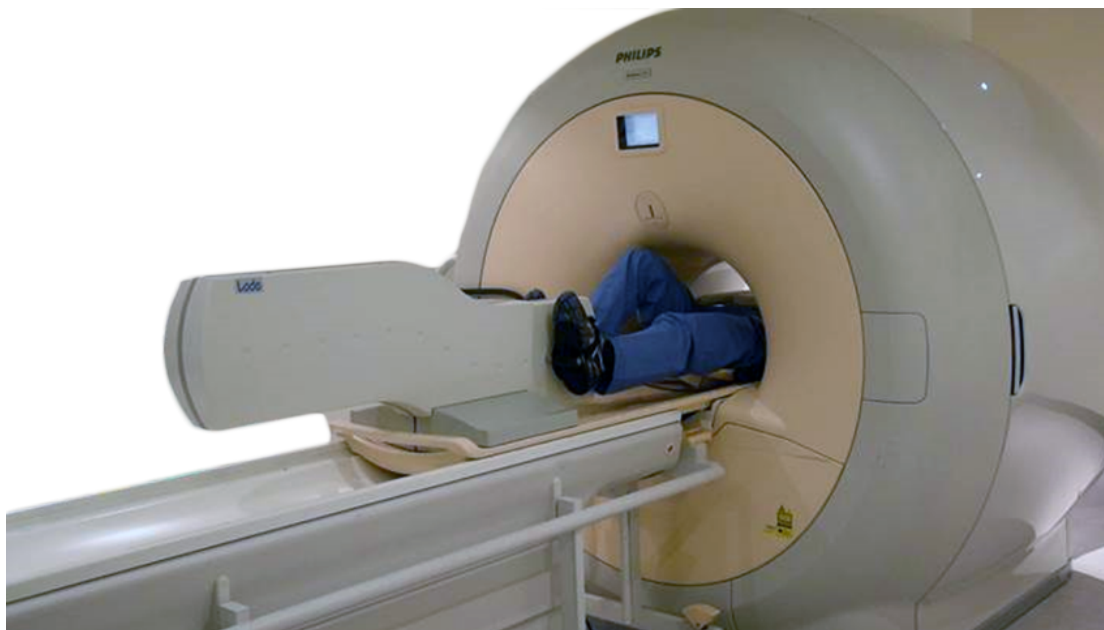
Figure 3.1: Set up of cycle ergometer with a subject inside the scanner.
