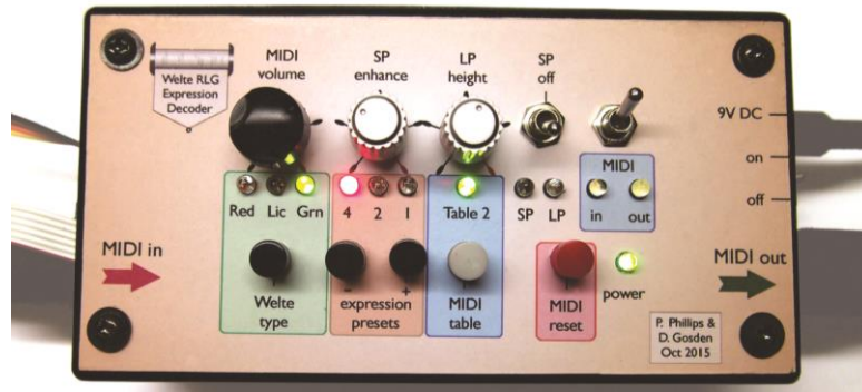
Figure 4.8 Microprocessor-based expression decoder for all types of Welte rolls
