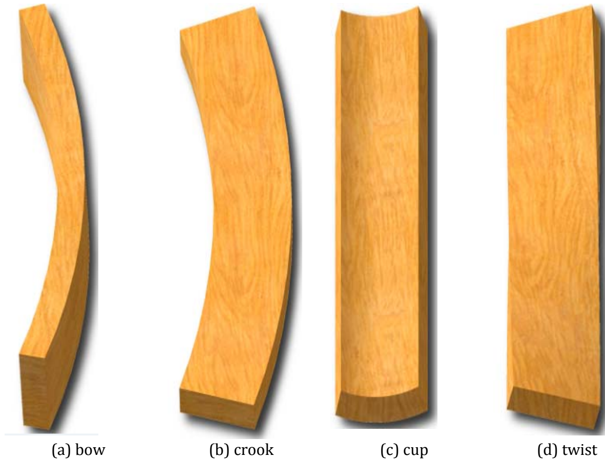
Figure 3.1. Different types of wood warping due to drying (Wengert and Meyer, 1993).
