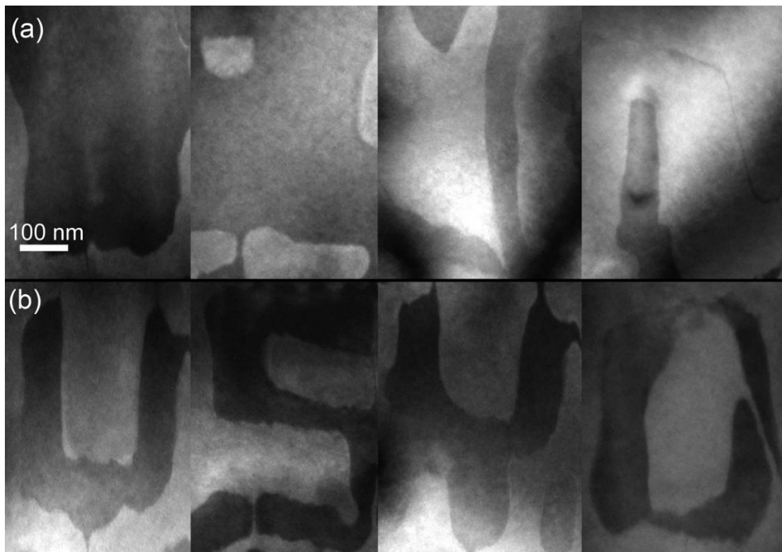
Figure 3-10 (a) Initial domain configurations in four areas before e-beam illumination. (b) Letters U, S, Y and D were written on the areas in (a) via e-beam illumination.
