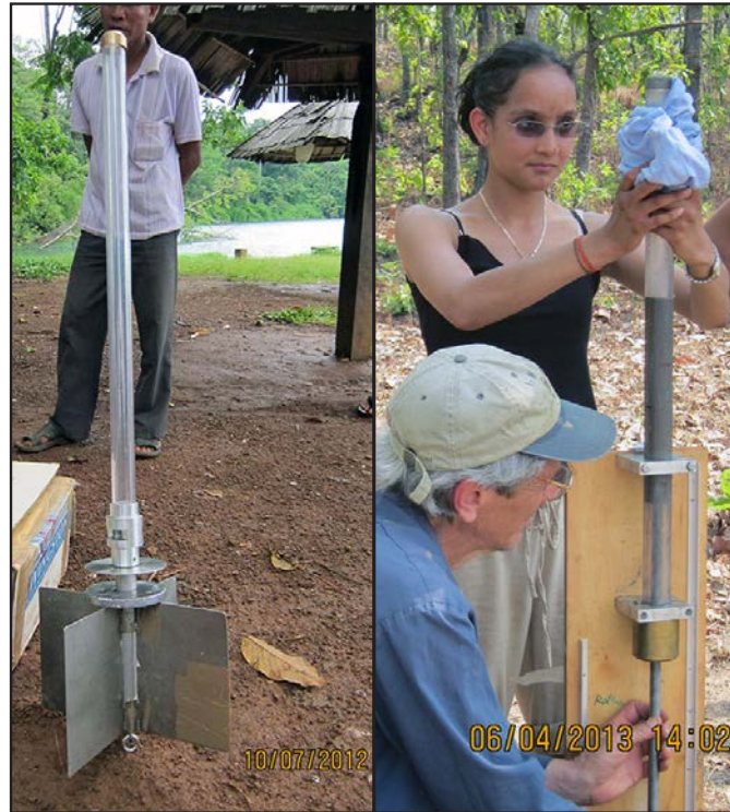
FIGURE 5.2: Photographs of miniature gravity corer (L) and sediment extruding device (R).
