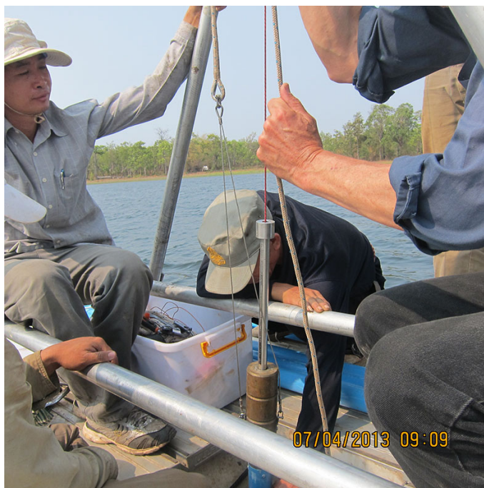
FIGURE 4.3: PVC core barrels being hammered into the sediment using percussion coring techniques.
