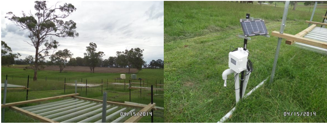
Figure S5. 4. Experimental set up (left picture) and data logger connected to solar panel (right picture).
