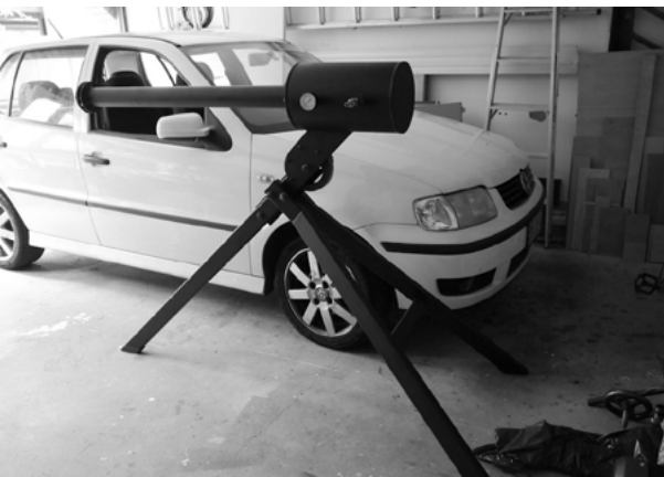
Development of colliding machines in 3 primary iterations, operated with winched spring power (top), compressed air and solenoid valves (middle), and high pressure compressed air with electromagnetic catches, separated into two working halves with individual pressure chambers (bottom). 2008-2016.
