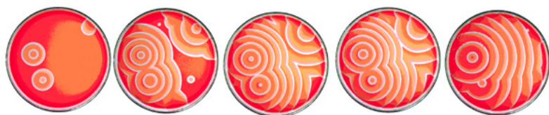
Progression of an oscillating BZ reaction taking place in a petri dish. Source - "Nonlinear Kinetics Group," accessed July 2, 2016, http://www1.chem.leeds.ac.uk/People/SKS/sks_research/sks_group_page.htm .
