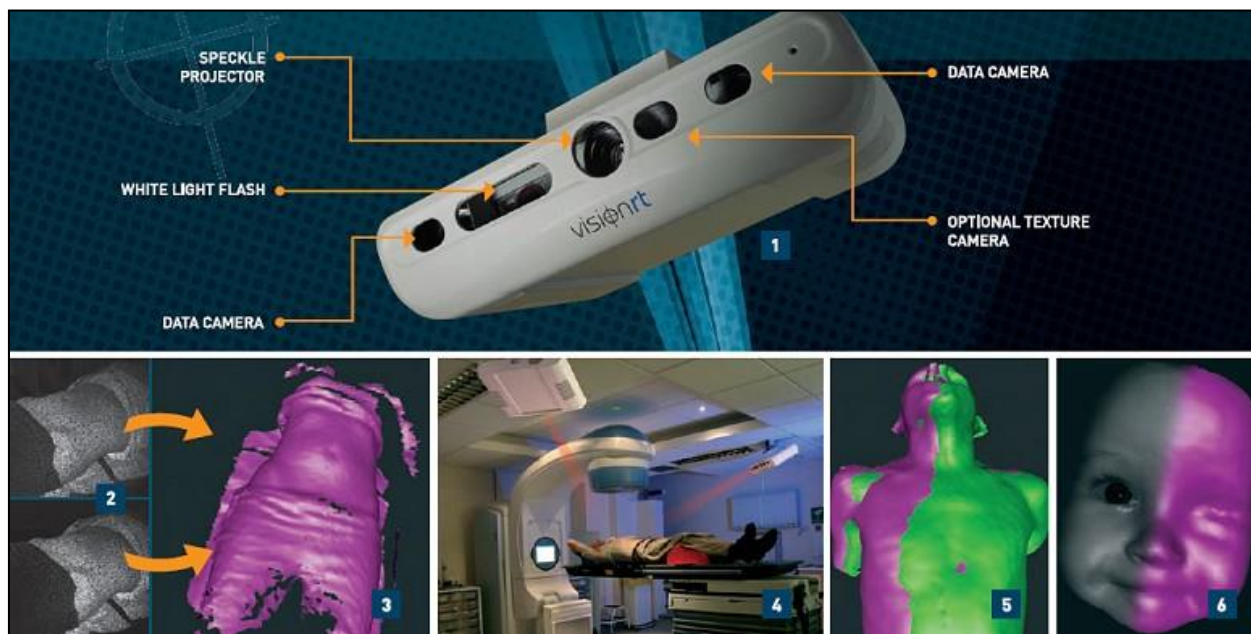
Figure 1-11. VisionRT AlignRT camera and examples of surface images. 86
