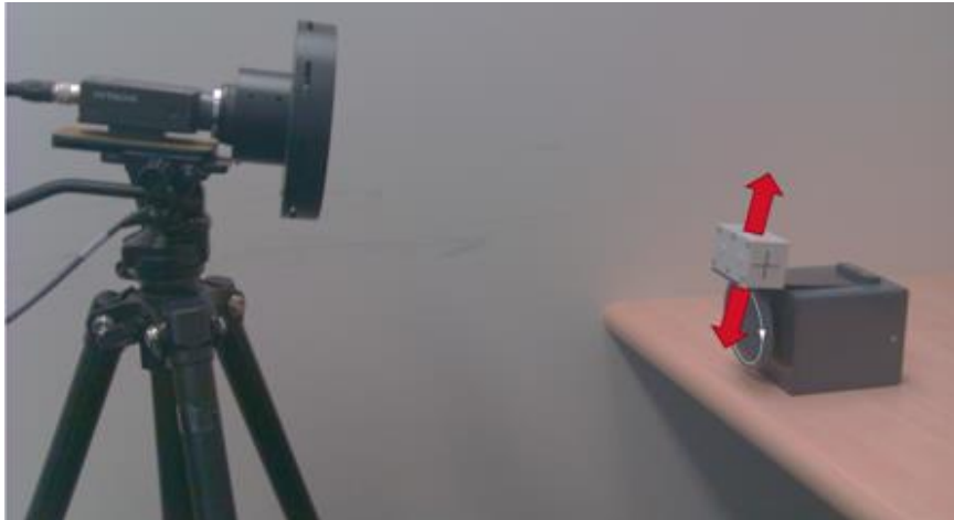
Figure 7. The RPM system: an IR camera tracking the marker block at a rate of 30 Hz.
