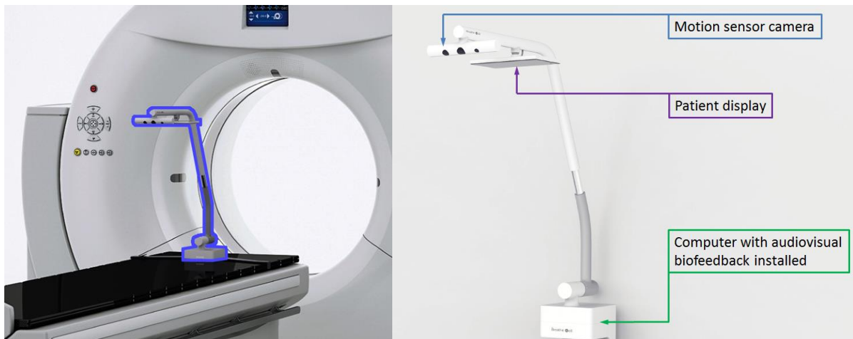
Figure 6-4. Audiovisual biofeedback product concept design, highlighted on the CT couch on the left, and components indicated on the right. Images courtesy of DESIGN + INDUSTRY Sydney. 26
