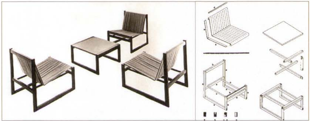
Figure 7.34 (left) The India lounge. Figure 7.35 (right) Exploded axonometric drawings to explain the construction technique 207
