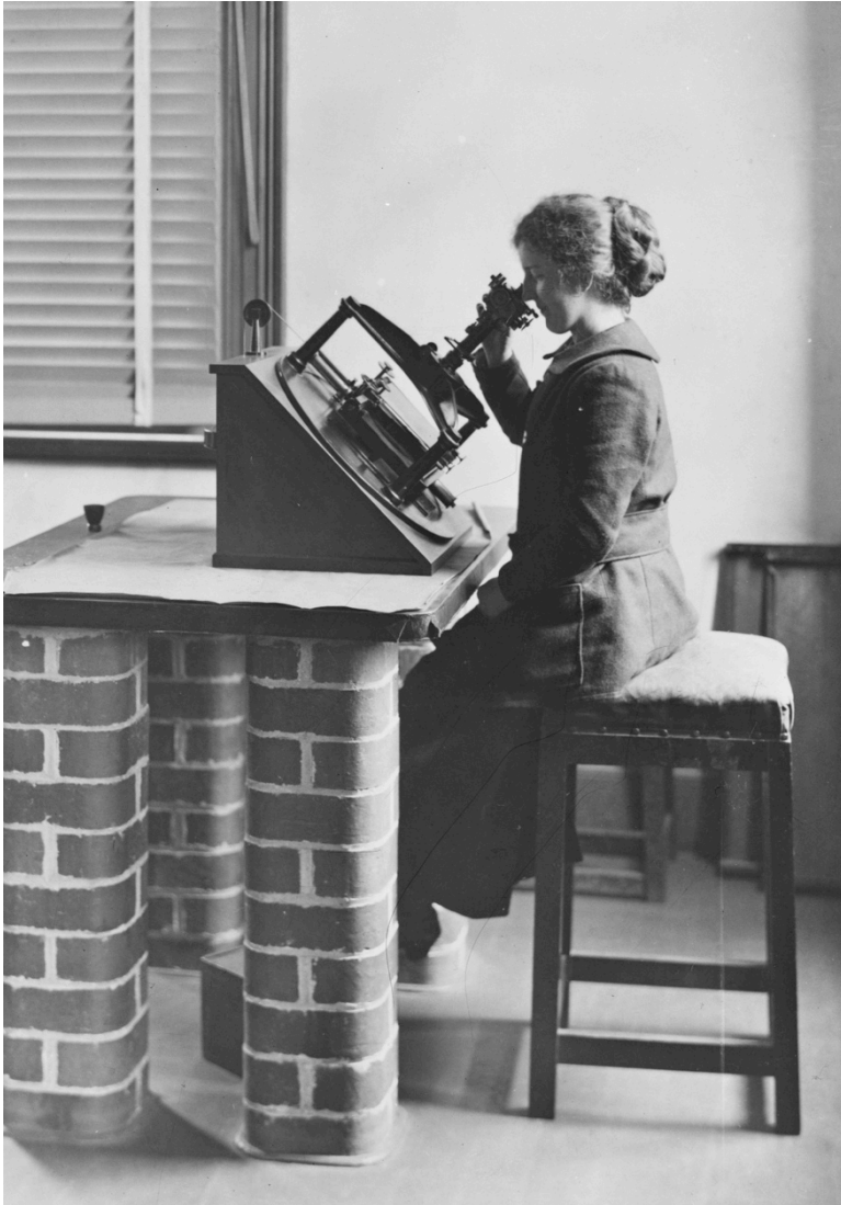
Figure 46: Melbourne Observatory star measurer using the 'Repsold' micrometer (Collection Museum Victoria).
