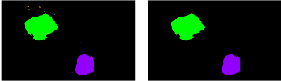
Figure 2-9 Detail of a two aggregates image segmentation process, different colours represent different labels.
