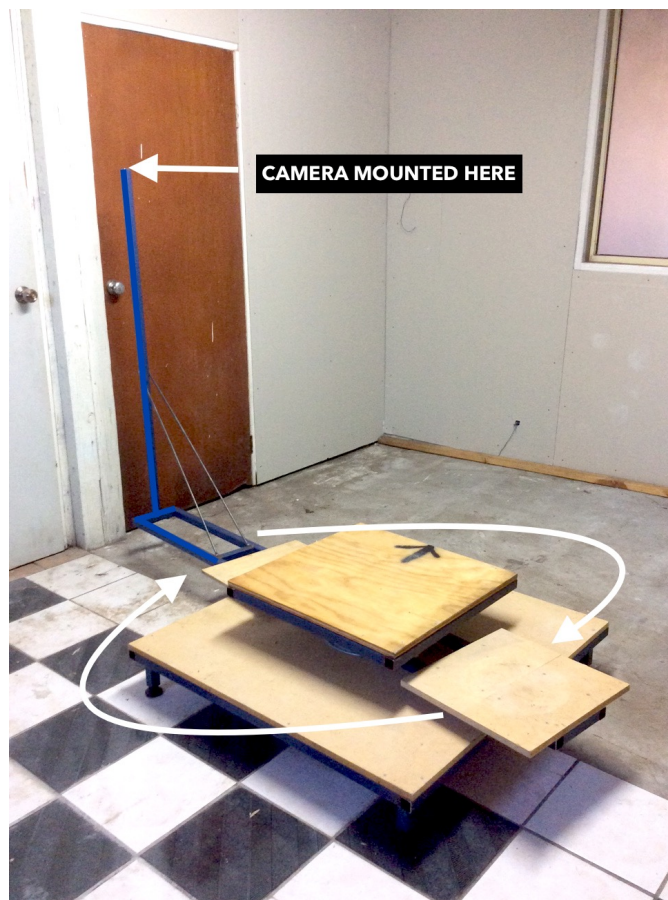
Fig33. James Nguyen 360-DEGREE ARC CAMERA RIG 2014. Rig mounted on Lazy Suzan mechanism and plywood and steel platform.
