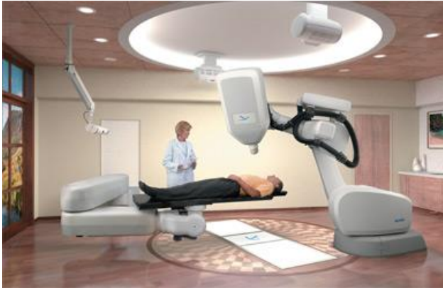
Figure 2-13. A compact linear accelerator, a computer-controlled arm and patient in a Cyberknife system.
