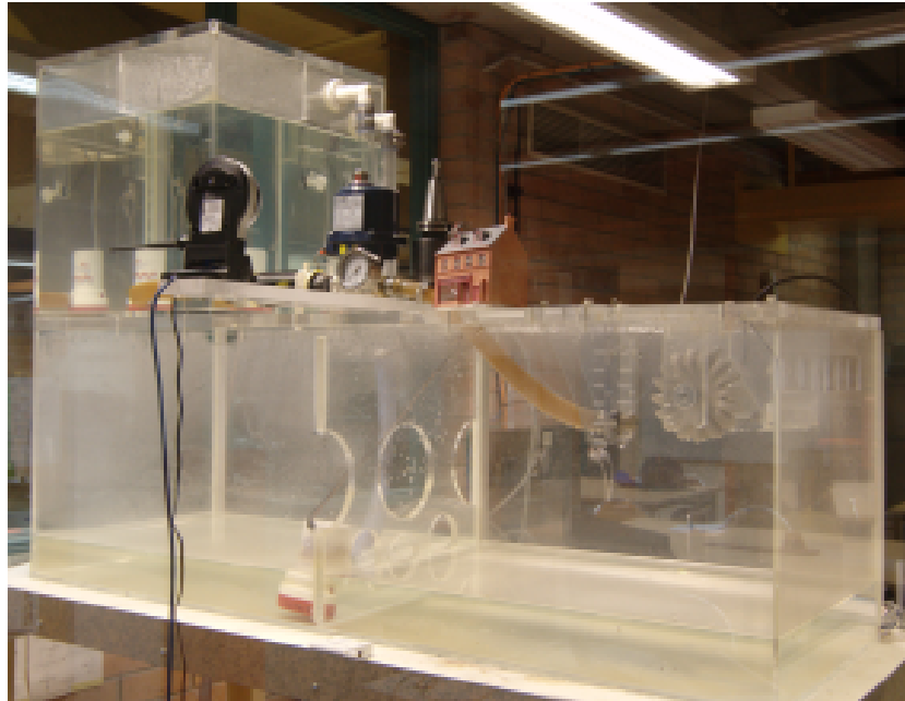
Figure 2.3: UTS remote hydroelectric energy laboratory equipment
