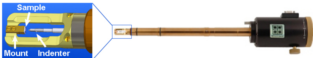
Figure 2-4 PI 95 TEM PicoIndenter holder for usage in JEOL TEMs [201].
