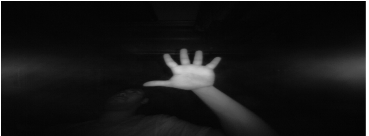
Figure 2.7: Raw Image from Leap Motion Controller
