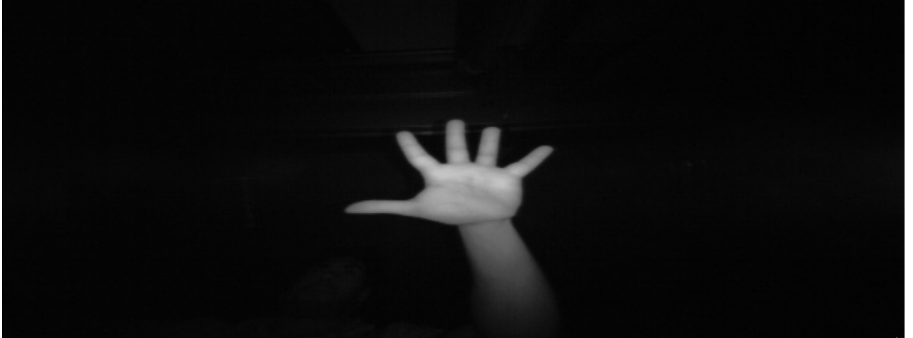
Figure 3.2: Raw Hand Image from Leap Motion sensor.
