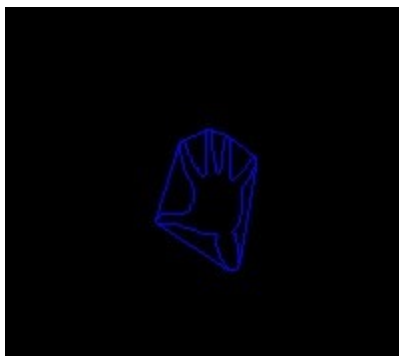
Figure 3.9: Sample Image displaying Hand Contour and Convex Hull.
