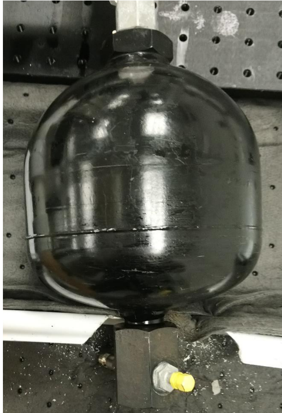
Figure 16: Diaphragm accumulator mimicking left ventricular function.
