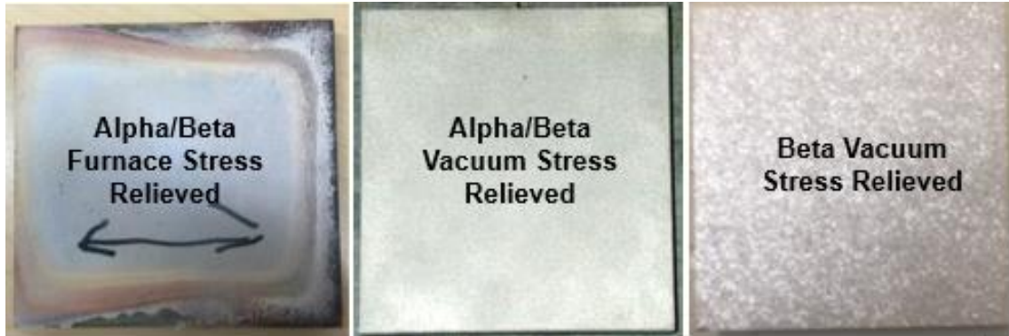
Figure 17: Substrate surface finish after each heat treatment procedure
