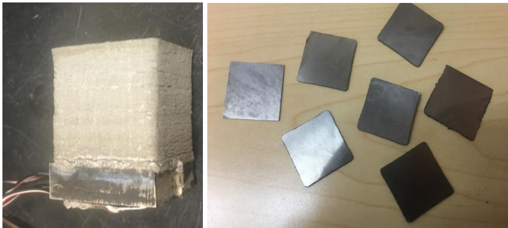
Figure 32: AM sample prepared for layer removal method (left) and cut AM slices during the procedure (right)
