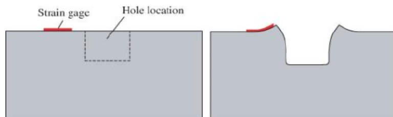
Figure 10: The outcome of the hole drilling procedure removing tensile residual stress on the surface [51]
