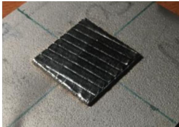
Figure 23: As-received substrate with 25.4 mm x 25.4 mm x 1.6 mm SLM deposit
