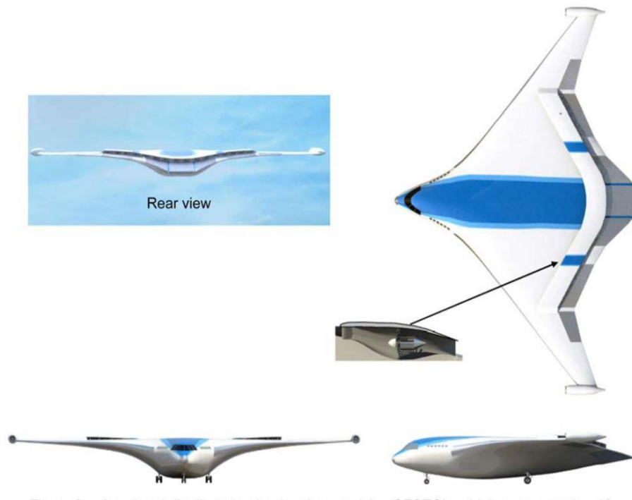
Figure 4: A BWB N+3 Turboelectric Distributed Propulsion Aircraft [10]
