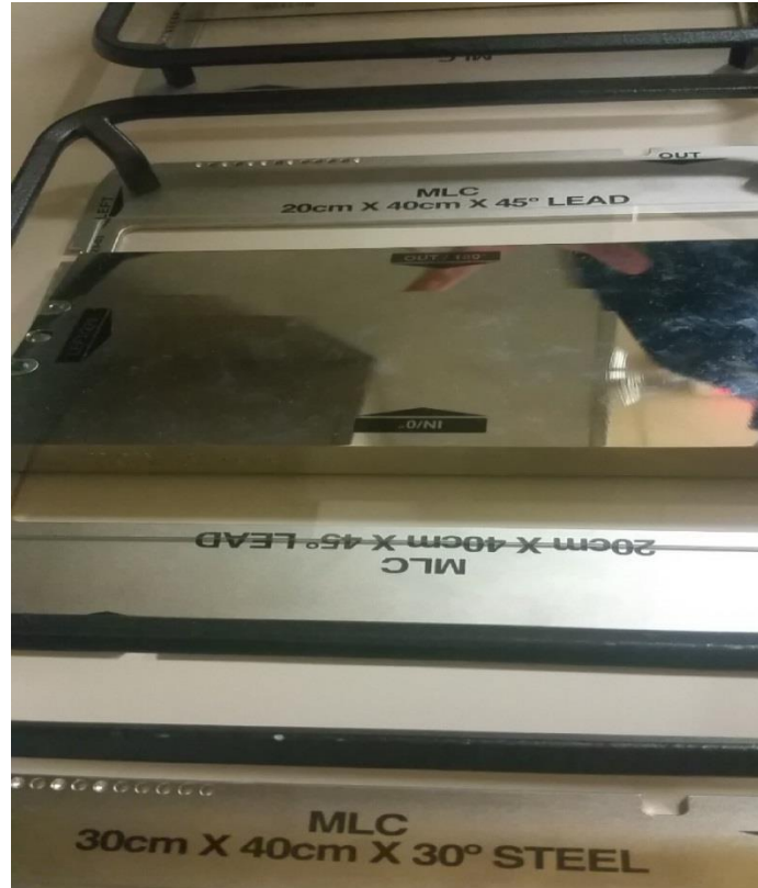
Figure 6. Physical wedges of the angle of 30° and 45° used in this study (original by author)
