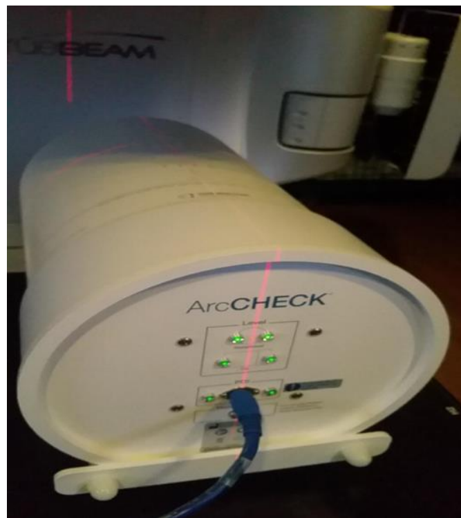
Figure 7. The ArcCHECK ® connected with laser sensor to assure positioning at the target point of the TrueBeam. (original by author)
