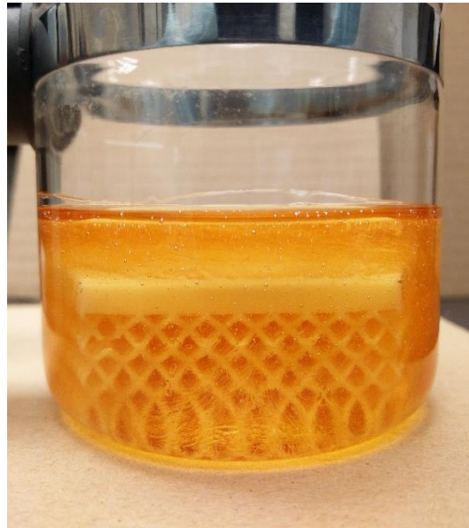
Figure 4.12 Specimen immersed in resin and set for curing.
