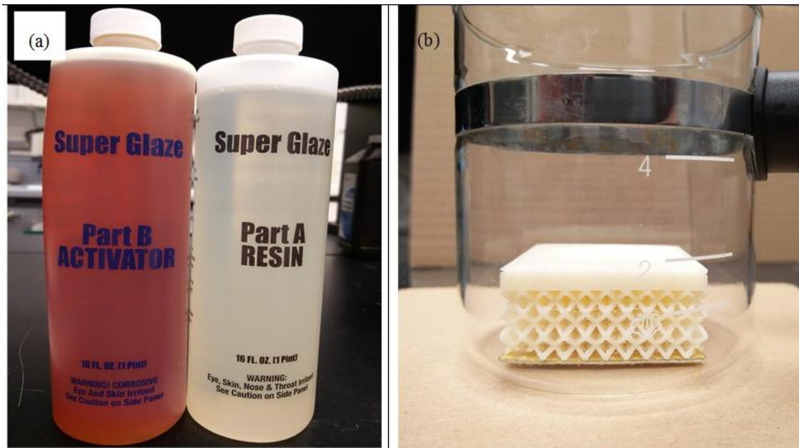
Figure 4.10 (a) Parks Resin, (b) Impact tested sample placed in a beaker.
