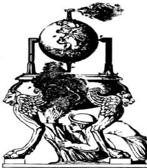
Figure 10: Heron's turning sphere invention [22]
