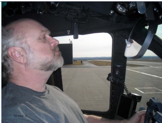
Figure 10. Subject placed at Cockpit DEP and then asked to move his head in order to see the HUD symbology.
