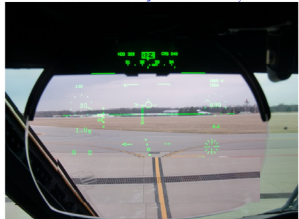
Figure 7. View of combiner when sitting in CDEP with a 25% loss of visible symbology (most common). Some subjects experienced a total loss of visible symbology.
