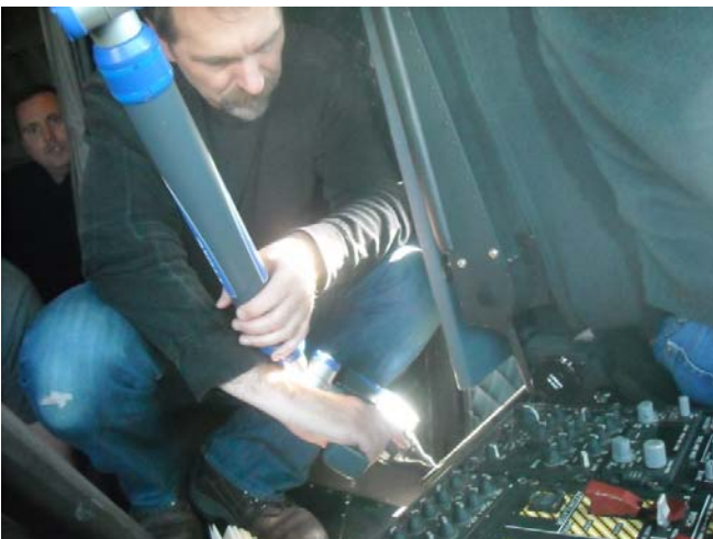
Figure 2. Installed FARO Arm for cockpit and subject digitization.
