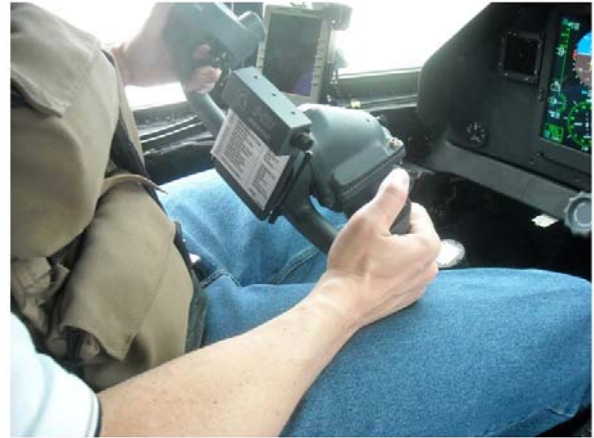
Figure 11. Yoke control interference was SEVERE when subject eye was placed in HUD Eye Box - 18 out of 19 subjects FAILED (with Survival Vest on).
