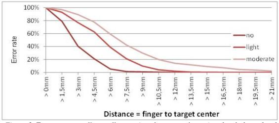
*Figure 2*: Error rate according to distance (touch to target in mm) and turbulence level for finger press
