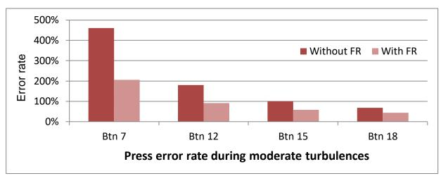
*Figure 7*: Error rate for various button sizes (in mm) with or without finger rest in moderate turbulence level.
