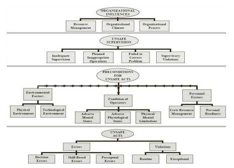
**Figure 1. The HFACS Framework.** Adapted from the "Human error approach to aviation accident analysis: The human factors analysis and classification system" by Wiegmannn, D. A., & Shappell., S. A. (2003). Burlington, VT: Ashgate Publishing Limited.
