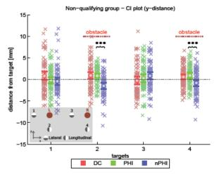
Figure 5: Distance in y-direction between reach and intended target, for the Q-group (n=5). Each cross represents the result of one trial, while the circles show the mean of all trials and the error bars indicate the 95% confidence intervals. Significance is denoted by "•", "••" and "•• •", representing  $p \le 0.05$ ,  $p \le 0.01$  and  $p \le 0.001$ , respectively.
