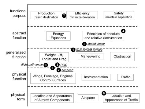
Figure 1: Abstraction Hierarchy for tactical navigation in the vertical plane.
