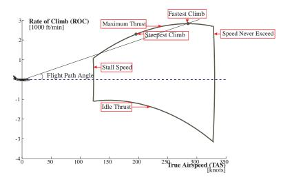
Figure 2: Performance envelope of the Cessna Citation I, in TAS/ROC state space.
