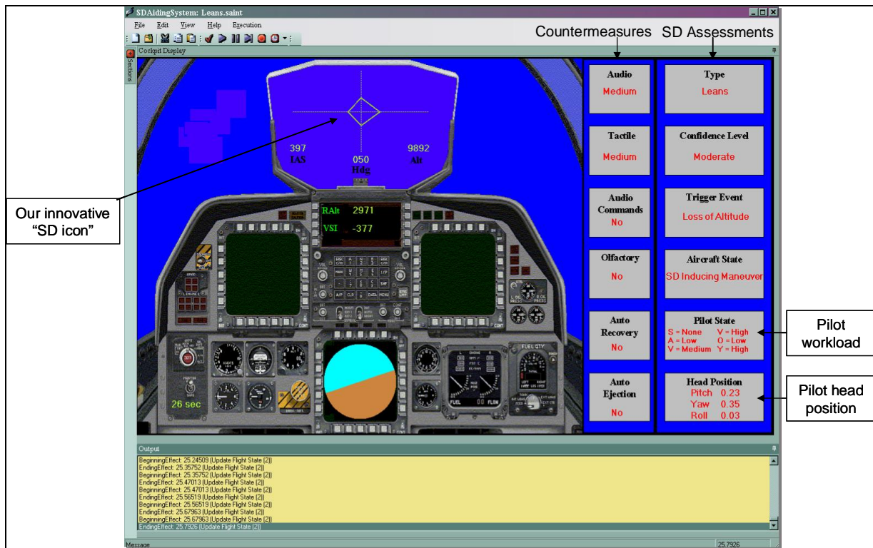
Figure 4. Simulated cockpit display used to evaluate SOAS. The Icon is depicted on the HUD, commanding a mild right roll. The boxes to the right are not part of the pilot’s display, but represent running parameters of the SOAS model, which would be responsible for triggering different countermeasures.
