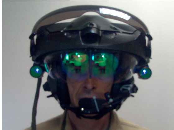
Figure 3. Topowl® Helmet used in the Tigre has side sensors thus qualifying as a Type II night vision device.
