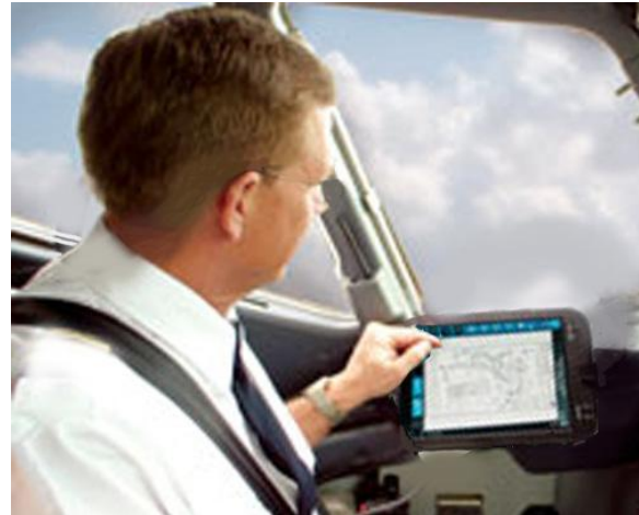
Figure 1. Approximate location and configuration of the touch screen during EFB testing
